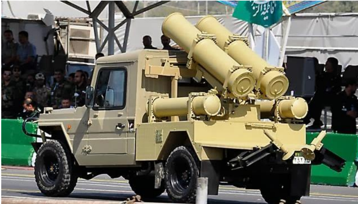
Figure 1.16 A twin-barrelled 333 mm self-propelled spin-stabilised rocket artillery system (photo credit: Hossein Fatemi/FARS News Agency).
