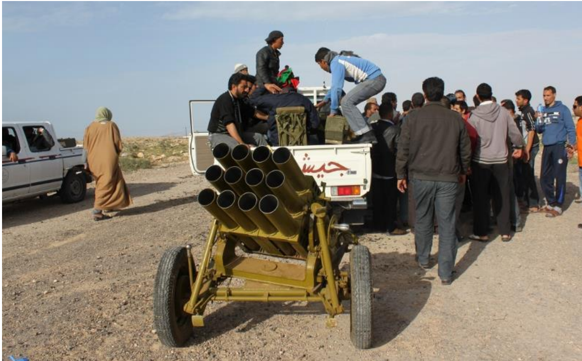
Figure 1.14 A multi-barrelled 107 mm towed spin-stabilised rocket artillery system (photo credit: Al Jazeera).
