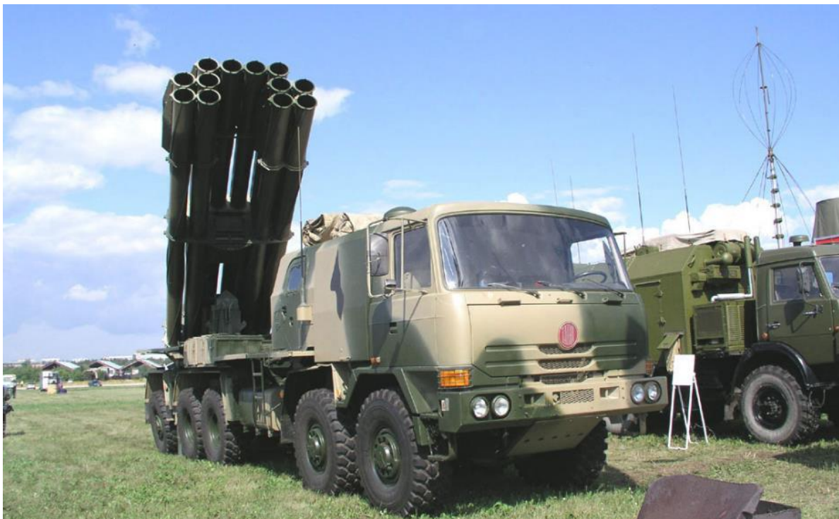
Figure 1.17 A multi-barrelled 333 mm self-propelled fin-stabilised rocket artillery system (photo credit: Military Today).
